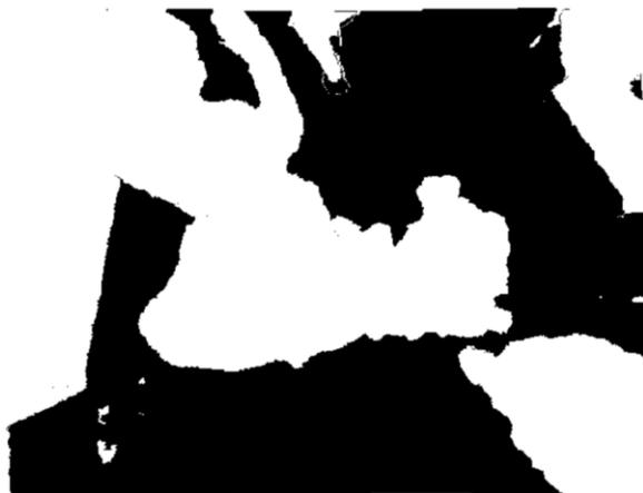
Figure 3: Movement detector applied to an image. White regions correspond to objects in movement.
