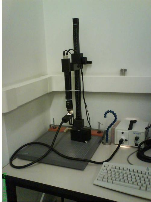
**Fig. 2.** Camera and lighting system used in the image acquisition.
