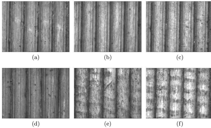
**Fig. 3.** Images of both classes 1 and 2. a, b and c with low roughness ( $R_a$  of 2.66, 2.77 and 2.82  $\mu m$  respectively) and d, e and f with high roughness ( $R_a$  of 3.65, 4.03 and 4.03  $\mu m$ )
