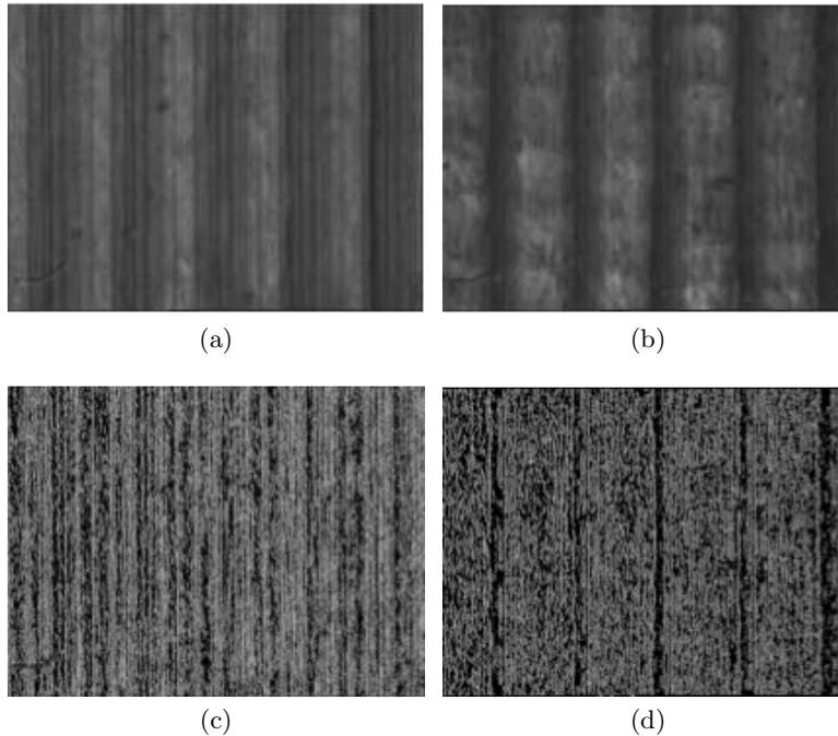
**Fig. 4.** a and b show original images with  $R_a$  of  $2.47 \mu m$  -left- and  $4.33 \mu m$  -right-. c and d show the same images after filtering.
